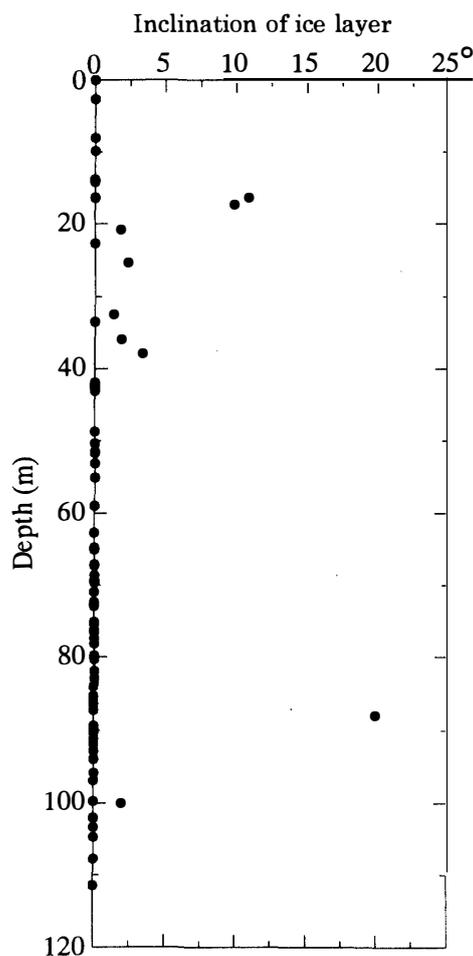
Fig. 4. Distribution of inclination of thin ice layers contained in shallow core.
