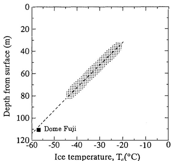
Fig. 9. Depth of the firn-ice transition layer versus ice temperature. The shaded portion shows the firn-ice transition layer at other places.
