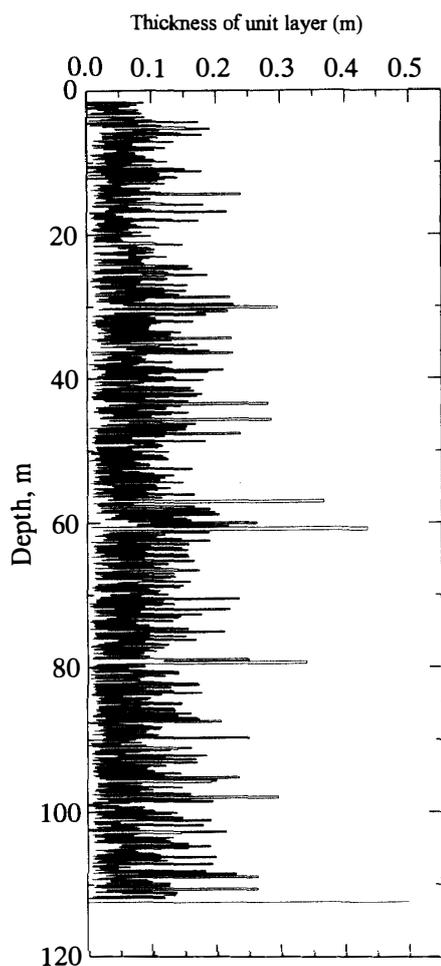
Fig. 3. Profile of thickness of unit layer obtained from observation of stratigraphy.
