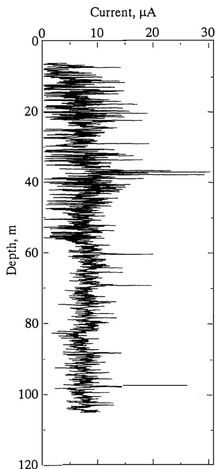
Fig. 8. ECM data of Dome Fuji shallow core.
