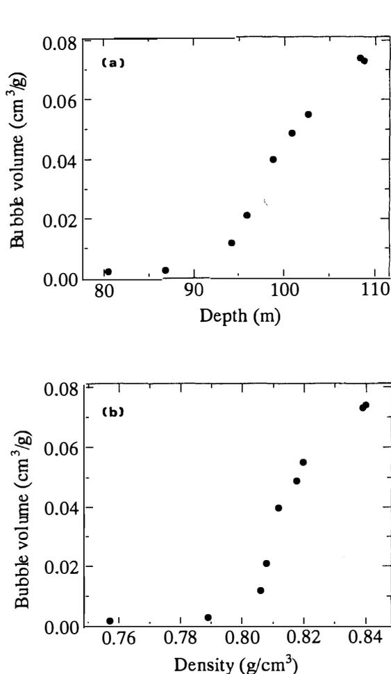
Fig. 7. (a) Relationship between air bubble volume and depth, (b) relationship between air bubble volume and density.
