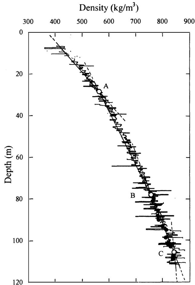
Fig. 2. Bulk density profile of Dome Fuji shallow core. Black dots are exact measured values.
