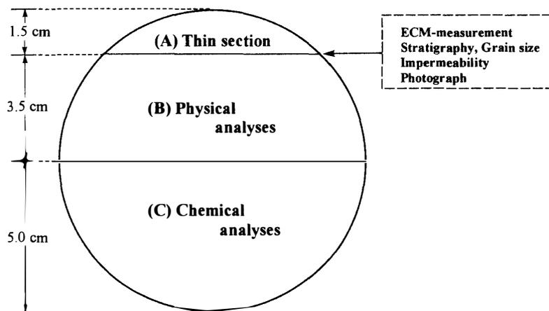
Fig. 1. Diagram of specimens cut for physical and chemical analyses for '93 Dome Fuji shallow core.
