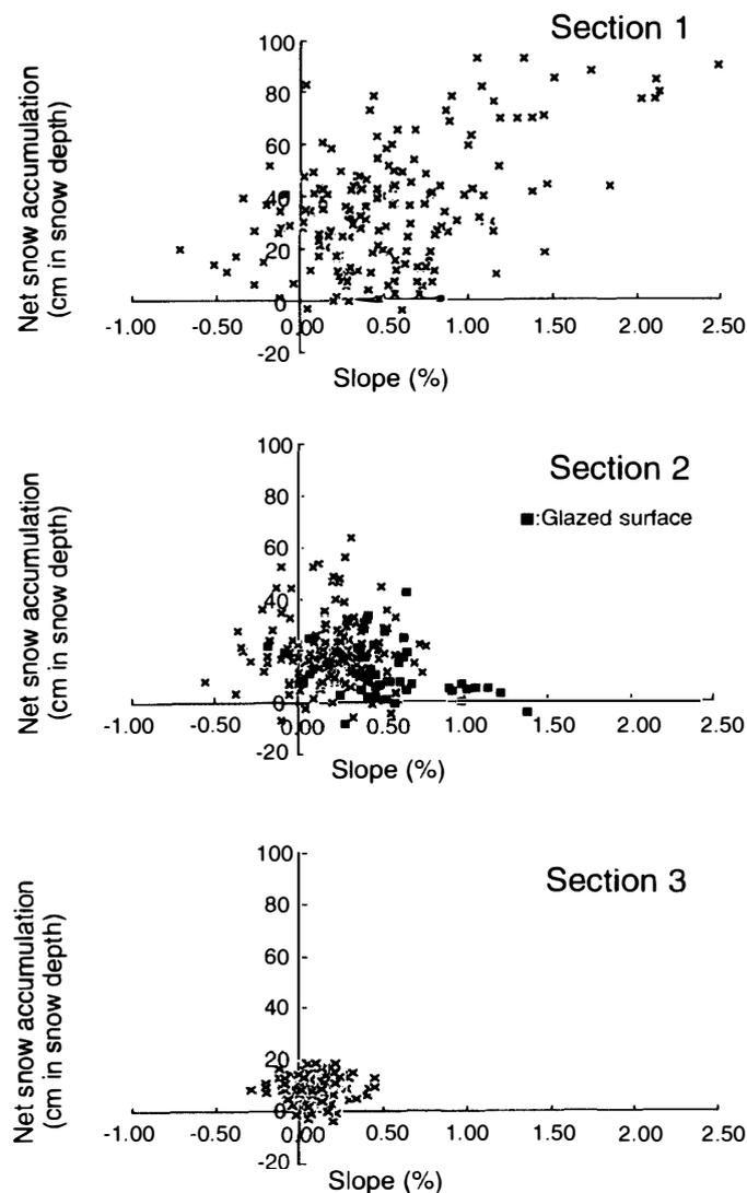
Fig. 4. Relationship between surface slope and net snow accumulation for Section 1, Section 2 and Section 3. Squares indicate the existence of glazed surface.
