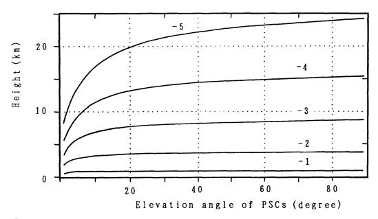
Fig. 2. The height of PSCs bottom and the elevation angle of the bright PSCs edge for sun elevation angles of -1, -2, -3, -4 and  $-5^{\circ}$ .
