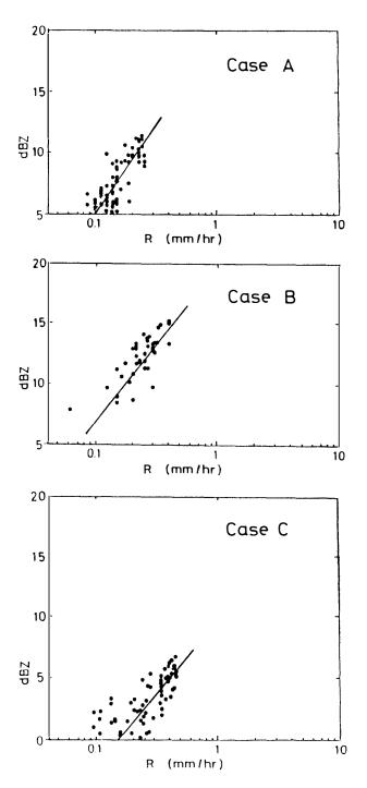
Fig. 2. The relationship between snowfall rate and radar reflectivity factor observed at Syowa Station (Case A: October 25, 1989, Case B: July 1, 1989, Case C: May 22, 1989).
