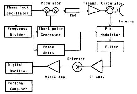
Fig. 2. Block diagram of a C-band radar for hidden crevasse detection with a very short pulse length.
