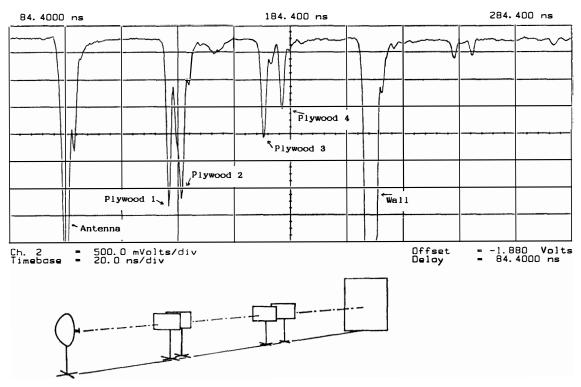
Fig. 3. Results of a preliminary experiment in a laboratory. Echoes of four targets made of plywood board are clearly detected.
