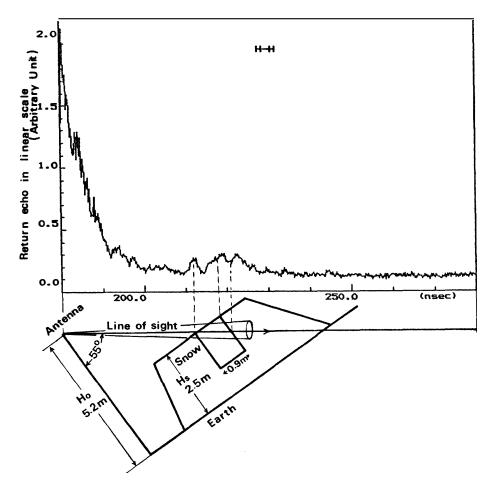
Fig. 4. Results of preliminary experiment to detect the walls of a pit dug in a snow pile. Two peaks which correspond to echoes originating from edges of the snow walls are detected.
