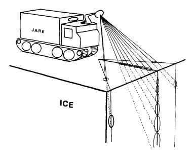
Fig. 1. Conceptual figure of a crevasse detection radar on a snowmobile which detects hidden crevasses by transmitting a short pulse to the snow surface and analyzing the echo signals with range-gate methods.
