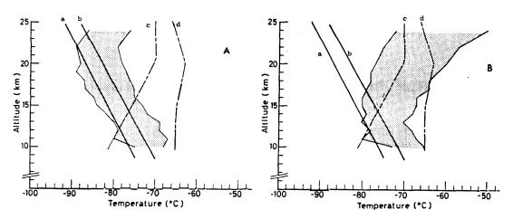
Fig. 1. The shaded area indicates the observed temperature range at Syowa Station (69°S, 40°E) in July 1985 (A) and in September (B). Lines a and b are frost-point temperature of pure water. Lines c and d are frost point of HNO<sub>3</sub>-H<sub>2</sub>O (50% weight) crystal.
