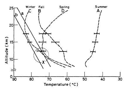
Fig. 1. Seasonal changes in temperature profiles measured at Syowa Station (69°00'S, 39°35'E). Curves A, B, C and D are the atmospheric temperatures which are half-monthly averaged; A: February 1–15 (summer), B: May 16–31 (fall), C: July 1–15 (winter), D: September 16–30 (spring). Frost point temperature for water vapor = 5 ppmv (curve a) and 10 ppmv (b) are compared.
