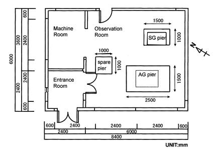
Fig. 1. Sketch of the gravity observation hut.
