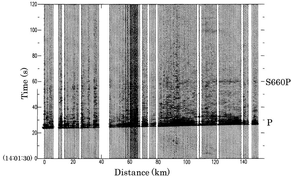
Fig. 3. Record section showing seismic waves of the Kermadec Is. event ( $m_b=4.5$ , depth=437 km). The vertical axis indicates relative time measured from Jan. 21, 2002, 1401:30.0 (UTC). We show here the original (no filter) traces with high signal-to-noise ratio. Signals during 20–30 s are composed of direct P and possibly reverberations in the ice sheet. Faint signals found in 50–60 s may be an S-P converted wave at the 660 km discontinuity just beneath the event (S660P).
