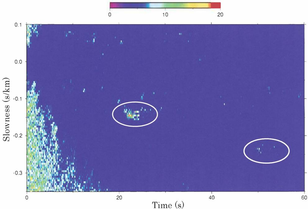
Fig. 9. Same as in Fig. 7b but for icequakes. Peaks corresponding to two obvious waves shown in Fig. 4 are indicated by white ellipses: peaks at (23 s,  $-0.135$  s/km) and (51 s,  $-0.235$  s/km). Note that high amplitudes found at the upper and lower left are artifacts caused by the PWS applied to zero-amplitude portions: since the zero amplitudes have the same value of phase components, a sum of the phase components should have a large value.
