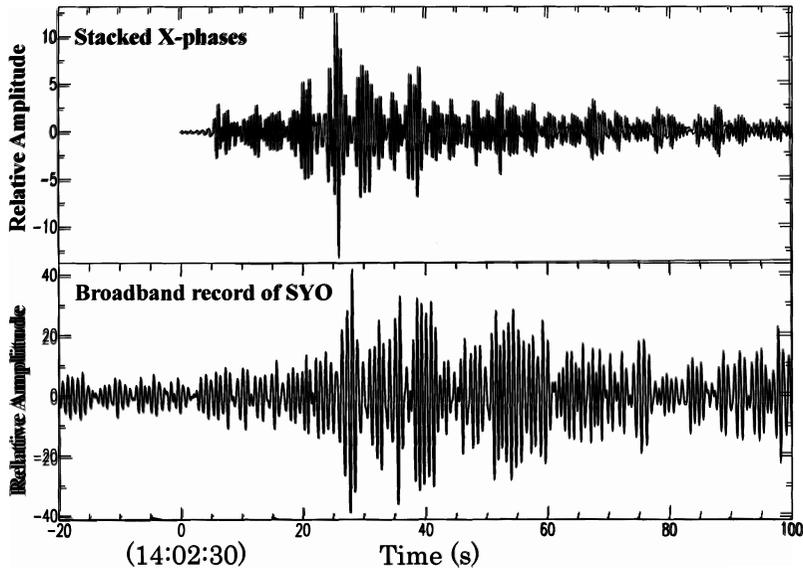
Fig. 13. Comparing the stacked trace of the X-phases (top) and a broadband record of SYO (bottom) after correction of the instrument response of the seismograph used in the JARE-43 experiments. Both traces are band-pass (1.0–2.0 Hz) filtered. The origin of the time axis (0 s) corresponds to 1402:30.0 (UTC).
