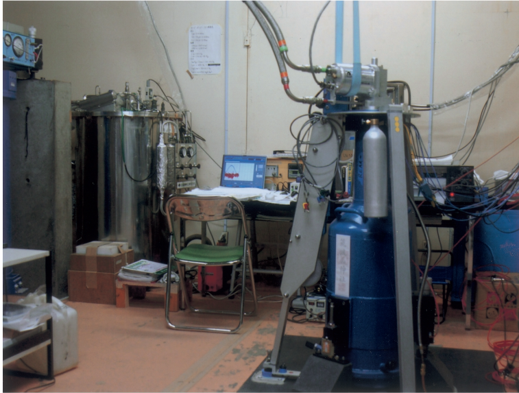
Fig. 7. The new SG CT (#043) is being installed in the gravity observation hut. Instead of the current pillar (left end of the photo), the tripod will support the 4K cryo-cooler, which is tentatively hung by the light-blue belt from the ceiling. The new CT (#043) will be moved to the pillar site after performance test. The photo was taken and sent by H. Ikeda (JARE-44).
