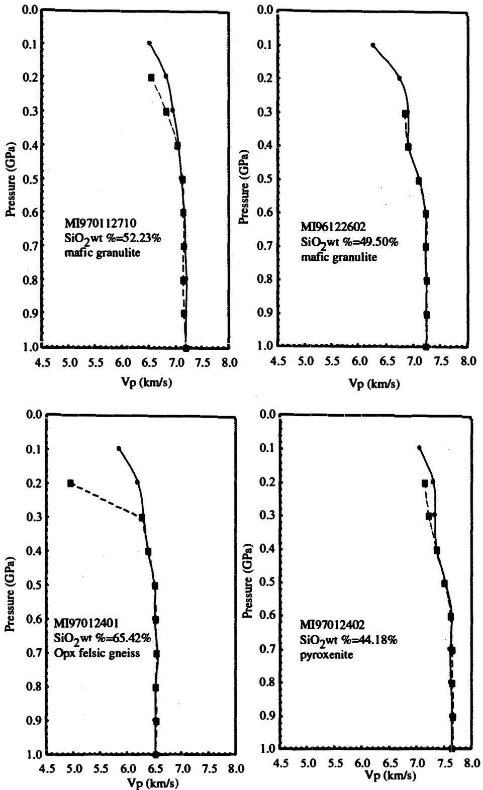
Fig. 5. P wave velocity versus pressure for all runs at 25°C. The broken line means  $V_p$  during pressurization and the solid line means during decompression.
