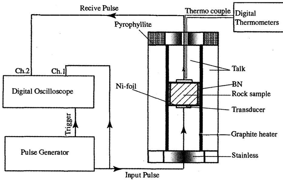
Fig. 2. High pressure cell assembly and the ultrasonic attachment.
