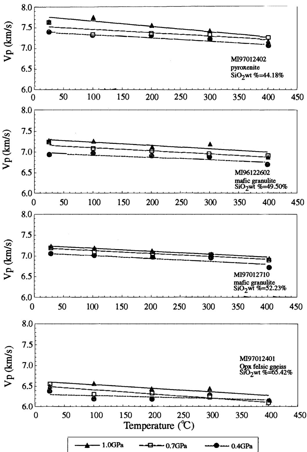
Fig. 6. Relation between P-wave velocities and run temperature. A solid triangle represents run temperature at 1.0 GPa; an open square represents run temperature at 0.7 GPa; and a solid circle represents run temperature at 0.4 GPa. Solid and broken lines are obtained by least square fitting.
