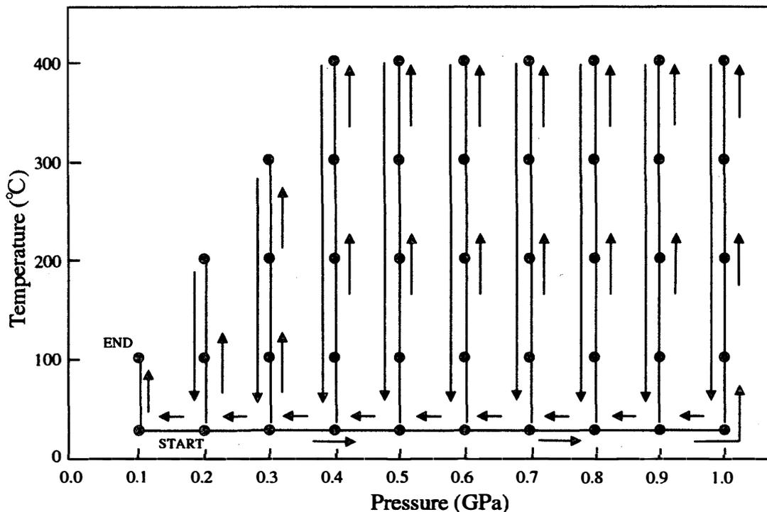
Fig. 4. Pressure-temperature path for a typical run.  $V_p$  was measured during pressurization from 0.1 GPa to 1.0 GPa at 0.1 GPa intervals, and subsequently was measured during decompression from 1.0 GPa to 0.1 GPa at 0.1 GPa interval and temperature from 25°C to 400°C.
