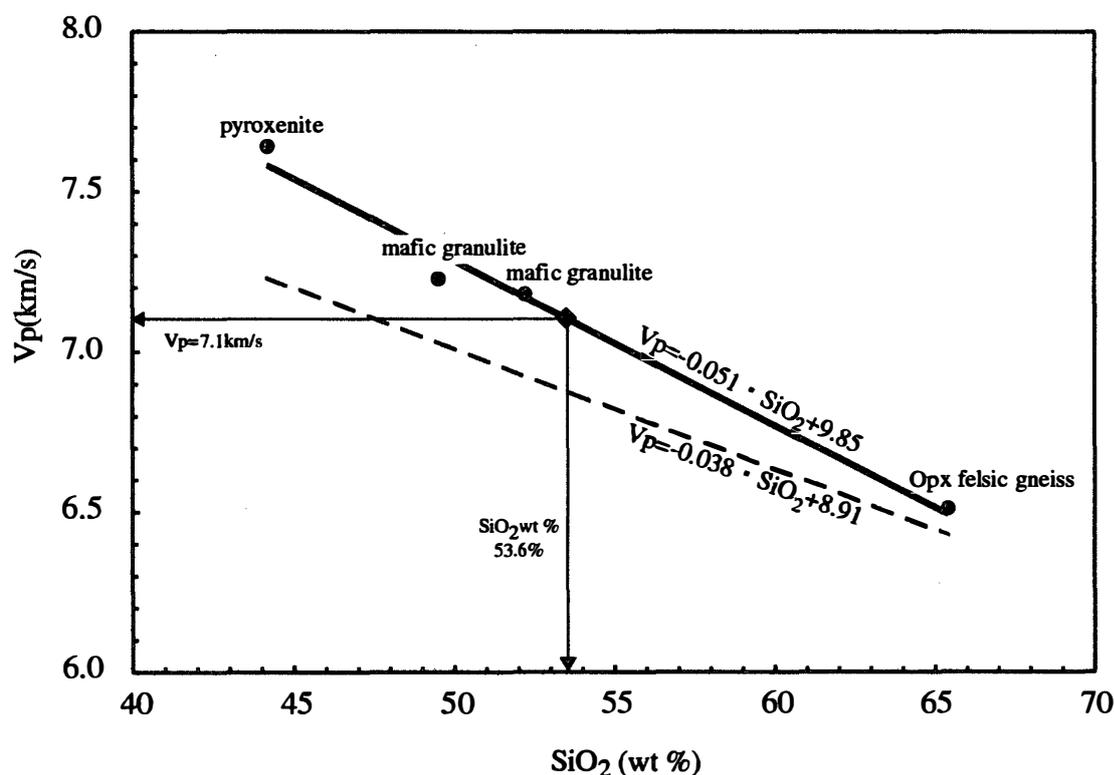
Fig. 8. *P*-wave velocities as a function of  $\text{SiO}_2$  wt% at 0.6 GPa and 25°C. Solid circles are present data. The solid line ( $V_p = -0.0513\text{SiO}_2 + 9.8469$ ) is a least square fitting. Broken line after Rudnick and Fountain (1995).
