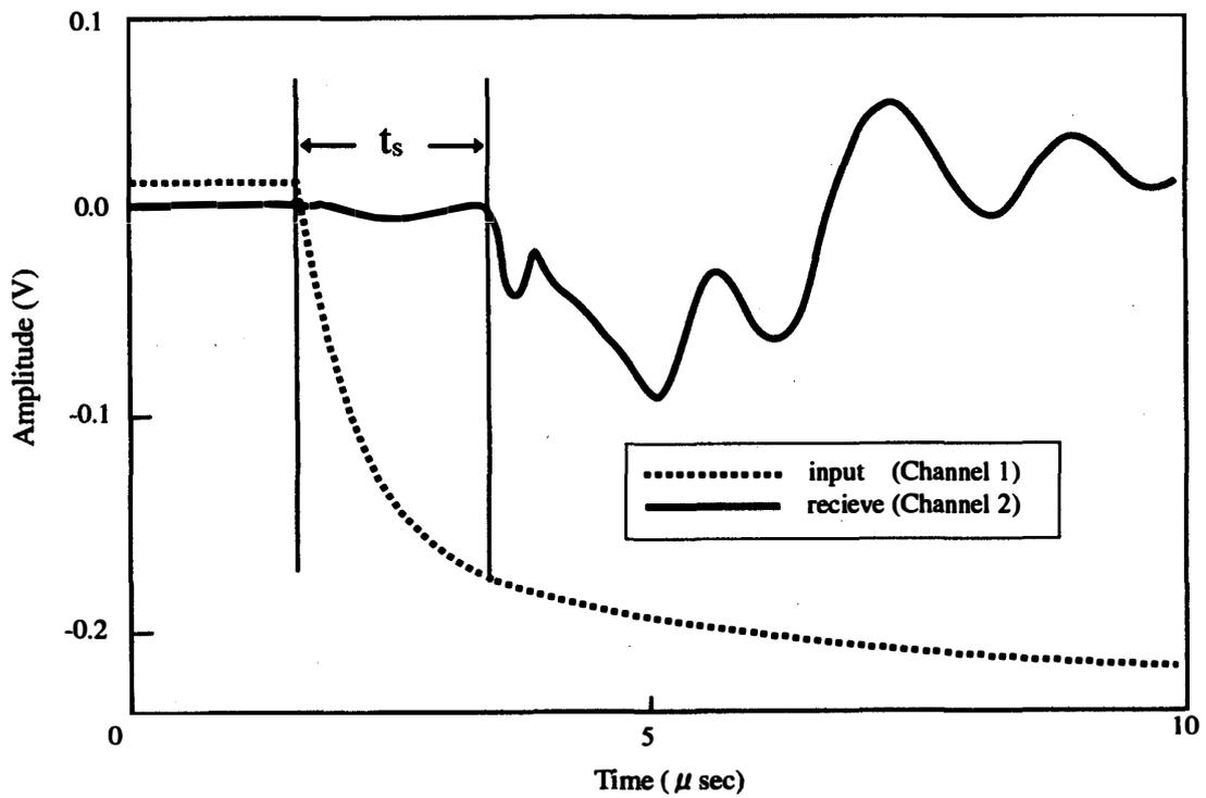
Fig. 3. Determination of travel times. The travel time  $t_s$  was determined by LSAR model. The  $t_s - t_0$  value is true travel time;  $t_0$  is the travel time when there is no sample.
