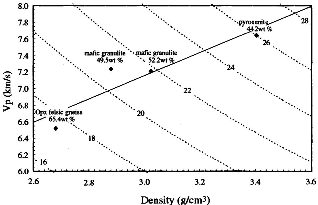
Fig. 7. Positive correlation between  $V_p$  and densities at 1.0 GPa and 25°C. Dotted lines shows constant acoustic impedance ( $\times 10^6$  kg/m<sup>2</sup>s<sup>-1</sup>).
