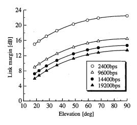
Fig. 3. Link margin and probe elevation.
