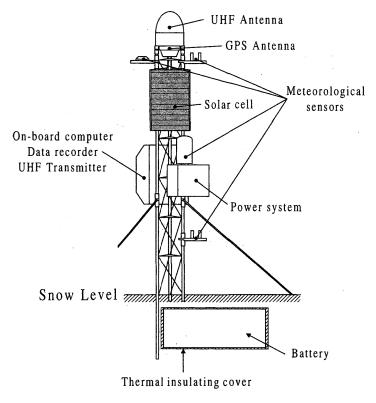
Fig. 4. Unmanned probe.
