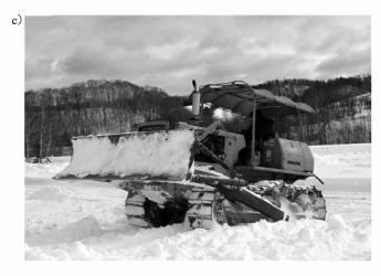
Fig. 3. (a) Rotary snowplow, (b) excavator, and (c) bulldozer used in the experiments conducted in 1998 and 1999.
