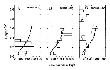
Fig. 9. Comparison of our final results for test fields A, B, and C obtained in 1999 with the profile of the wheeled C-130 shown in Fig. 8 (line with solid circles).
