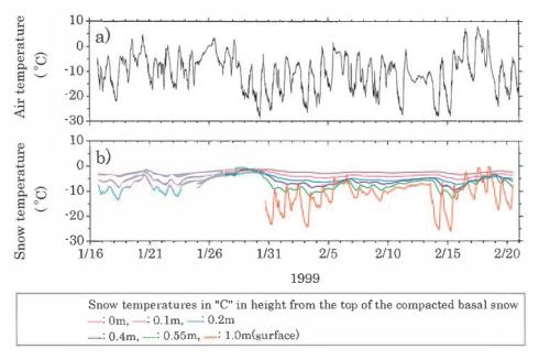
Fig. 4. Air temperature at a height of 1.5 m (a) and snow temperature (b) during the experiments in Rikubetsu. The heights from the compacted basal snow layer are shown.
