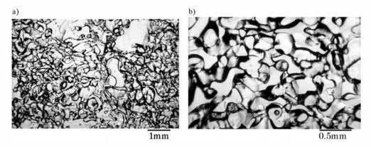
Fig. 7. Microscopic photograph of a hard compacted-snow layer. (a) Snow structure at a height of 0.2 m in test field B and (b) magnified view of the photograph shown in (a).
