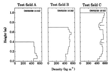
Fig. 6. Snow density distribution of test fields A, B, and C on February 20, 1999.
