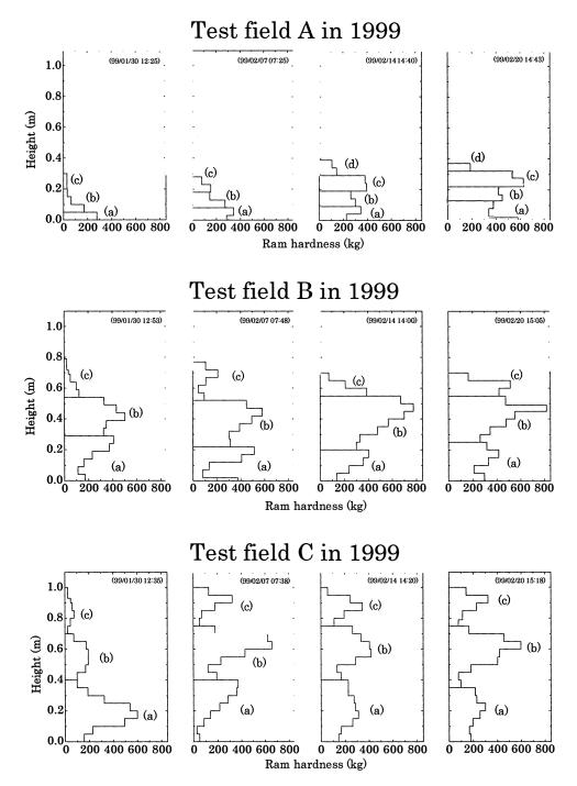
Fig. 5. Ram hardness profiles for test fields A, B, and C in 1999. Snow layers labeled (a) to (d) were deposited on January 16, 23, and 30 and February 7, respectively.
