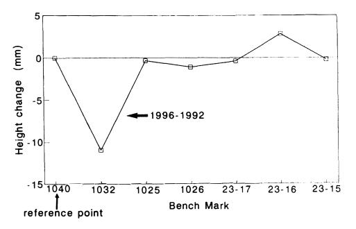
Fig. 2. Height changes between the measurements in 1992 and 1996.
