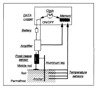
Fig. 4. Schematic sketch of the instruments.
