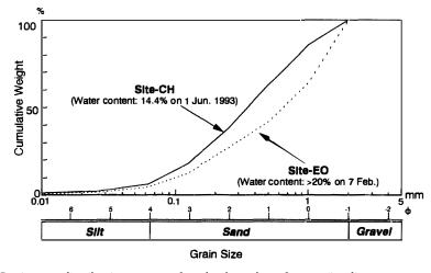
Fig. 3. Grain-size distribution curves for the less than 2 mm (in diameter) portion of the ground materials at the observation sites. The materials were collected from a few centimeters below the surface.
