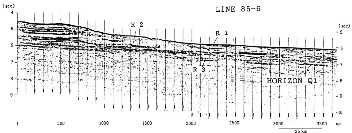
Fig. 7. Seismic reflection profile (Line TH85-6) showing the topographic boundary between the upper and the lower continental rise off Breid Bay, Dronning Maud Land.
