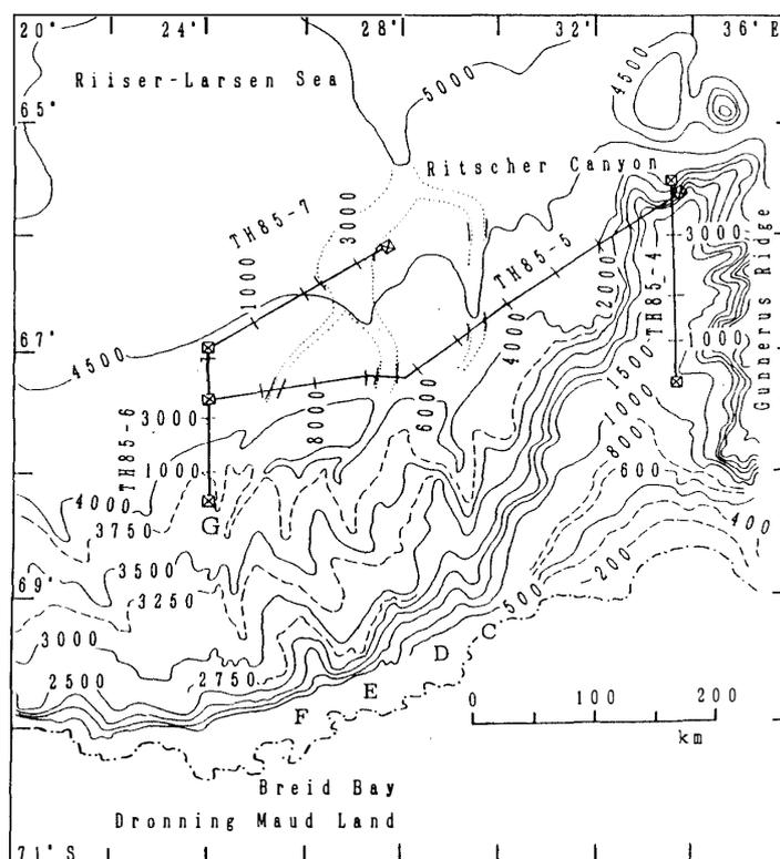
Fig. 1. Bathymetric chart of Ritscher Canyon off Breid Bay, Dronning Maud Land, East Antarctica. The locations of surveyed lines from TH85-4 to TH85-7 are shown. Alphabets (C to G) indicate tributaries of Ritscher Canyon. Depth interval is 500 m with subsidiary interval of 250 m.
