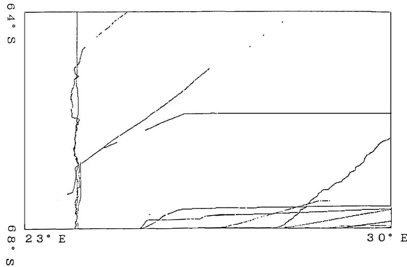
Fig. 2. Bathymetric survey lines collected during JARE-27 to -32 (except JARE-31) in the area between 23° to 30° E longitude and 64° to 68° S latitude.
