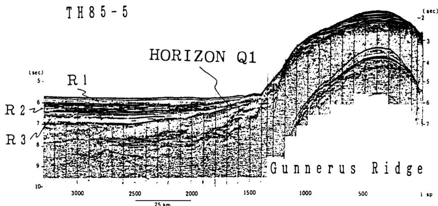
Fig. 6. Seismic reflection profile (Line TH85-5) crossing from Gunnerus Ridge to the lower continental rise of the Riiser-Larsen Sea.
