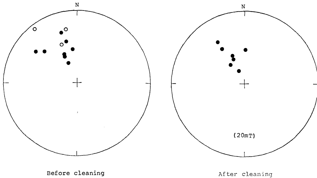
Fig. 8a. NRM directions before and after AF demagnetization, for Nils Larsenfjellet dolerites (site 12-2).
