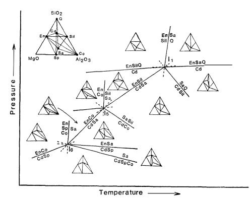
Fig. 1. P-T grid showing phase relations in MAS system. The univariant reactions En + Sil = Sa + Q and Cd + Sil = Sa + Q define the lower temperature stability limit of the assemblage sapphirine + quartz. HENSEN (1987) estimated P-T position of the invariant point I(1) at about 900-1000°C and 9-10 kbar.
