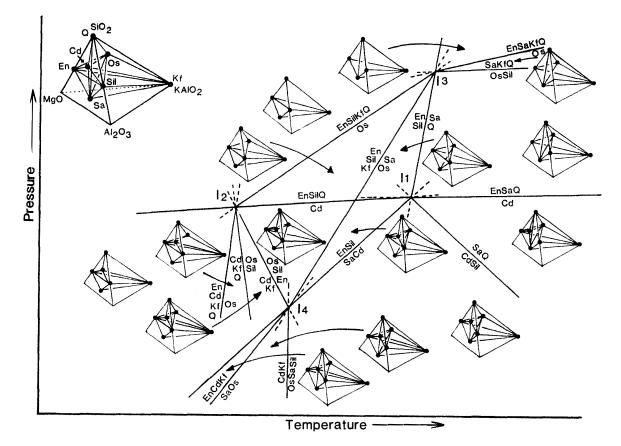
Fig. 2. P-T grid in KMAS system depicting the stability relations of osumilite in both quartzpresent and quartz-absent compositions under granulite facies metamorphic conditions. The invariant point 1(2) is located at temperatures lower than those for the invariant point 1(1), and osumilite-bearing assemblages can be stable at temperatures lower than those for sapphirine-quartz stability.
