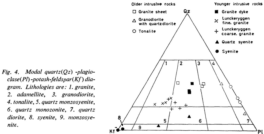
Fig. 4. Modal quartz(Qz) -plagioclase(Pl) -potash-feldspar(Kf) diagram. Lithologies are: 1. granite, 2. adamellite, 3. granodiorite, 4. tonalite, 5. quartz monzosyenite, 6. quartz monzonite, 7. quartz diorite, 8. syenite, 9. monzosyenite.
