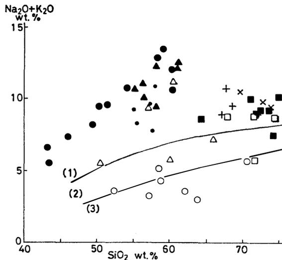
Fig. 8.  $\text{SiO}_2$ - $(\text{Na}_2\text{O} + \text{K}_2\text{O})$  diagram. Symbols same as in Fig. 5. Dots show the syenitic rocks from the Yamato and Belgica Mountains (KOJIMA *et al.* 1982; SHIRAIISHI *et al.*, 1983a). (1) Alkaline rock, (2) High-alkali tholeiite, (3) Low-alkali tholeiite.
