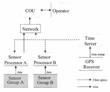
Fig. 3. Block diagramm of the sensor network MEDUSA-P.
