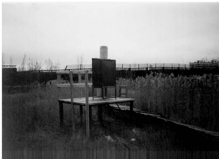
Fig. 2. Acid deposition sampler (winter).
