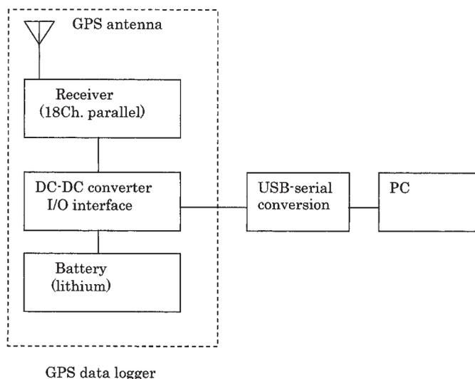
Fig. 1. Configuration of equipment. The computer is used to set the fixing schedule before an experiment and to read data after the experiment.
