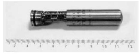
Fig. 2. An example of a data logger (Model M190-DT).
