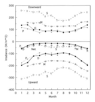
Fig. 3. Surface longwave radiation fluxes at Dome Fuji Station (D) in 1997, compared with those at three other Antarctic stations, Plateau (P; 1967), Mizuho (M; 1979) and Syowa (S; 1987).
