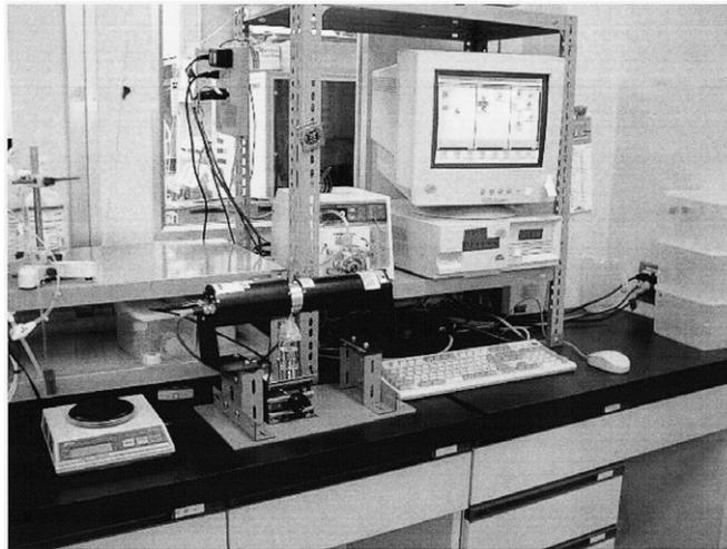
Fig. 1. A light scattering laser particle counter (Met One Model-211) located in a class 10000 clean room.
