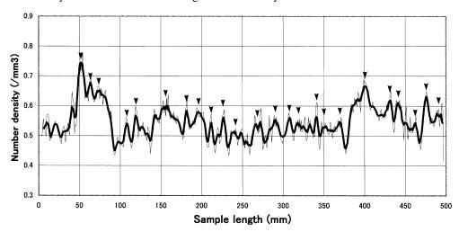
Fig. 3. The fluctuation of number density of air bubbles in direction of depth.
