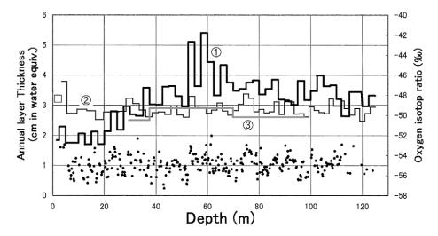
Fig. 2. Fluctuation of thickness of layer at near surface (line ①). Line ② is annual thickness obtained from D-J model. Another line ③ is the average accumulation rate from volcanic signals. □-mark is the accumulation rate obtained from the tritium signal. Small dots indicate values of the oxygen isotope ratio (δ<sup>18</sup>O).
