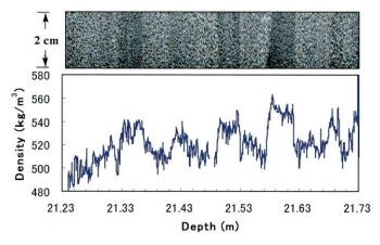
Fig. 1. An example of stratigraphy of the Dome Fuji shallow core, taken by X-ray scanning. Depth of the sample is 21.23–21.73 m.
