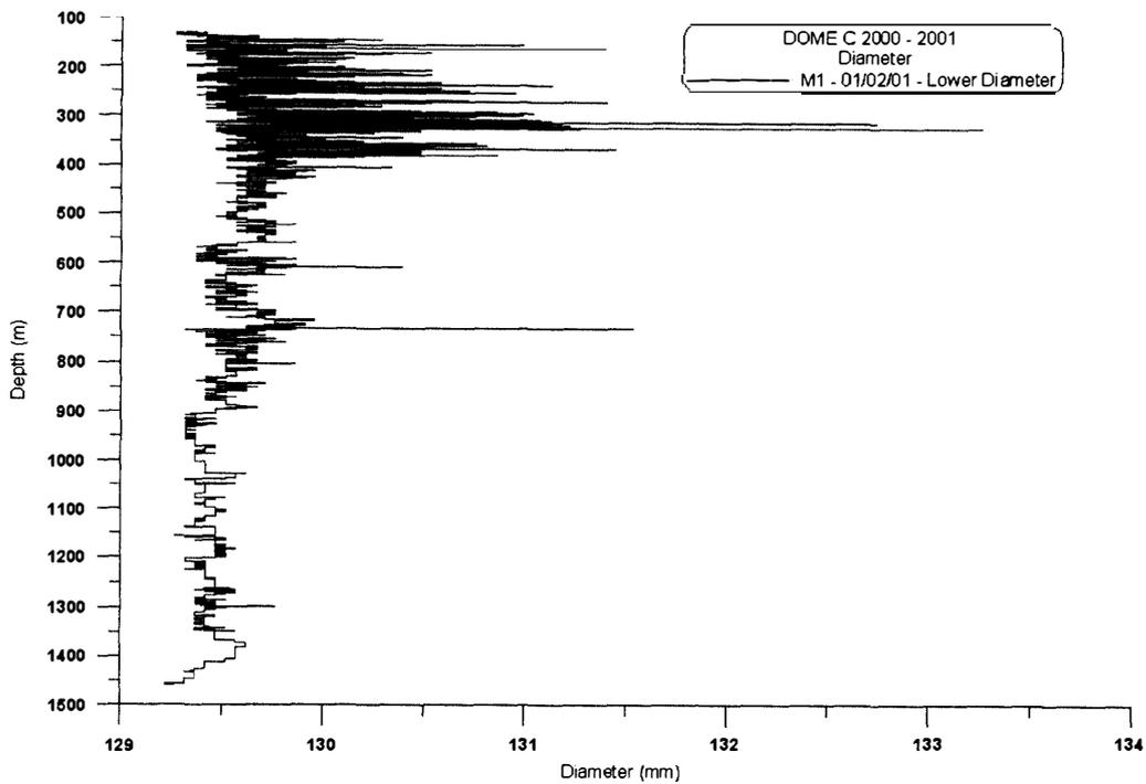
Fig. 9. The average diameter measured at lower pantograph of a borehole logger, in the Dome C second hole in 2001. The record of the measurements starts below the casing. We noticed many accidents at the beginning of the hole due to the mechanical problems. The second part shows a correct drilling operation.
