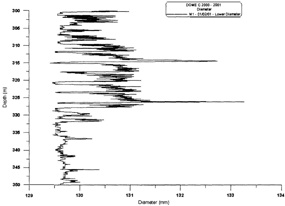
Fig. 8. The average diameter measured at lower pantograph, in the Dome C second hole in 2001. Diameter detail is between 300 and 350 m, when the drilling was disturbed by mechanical problems.
