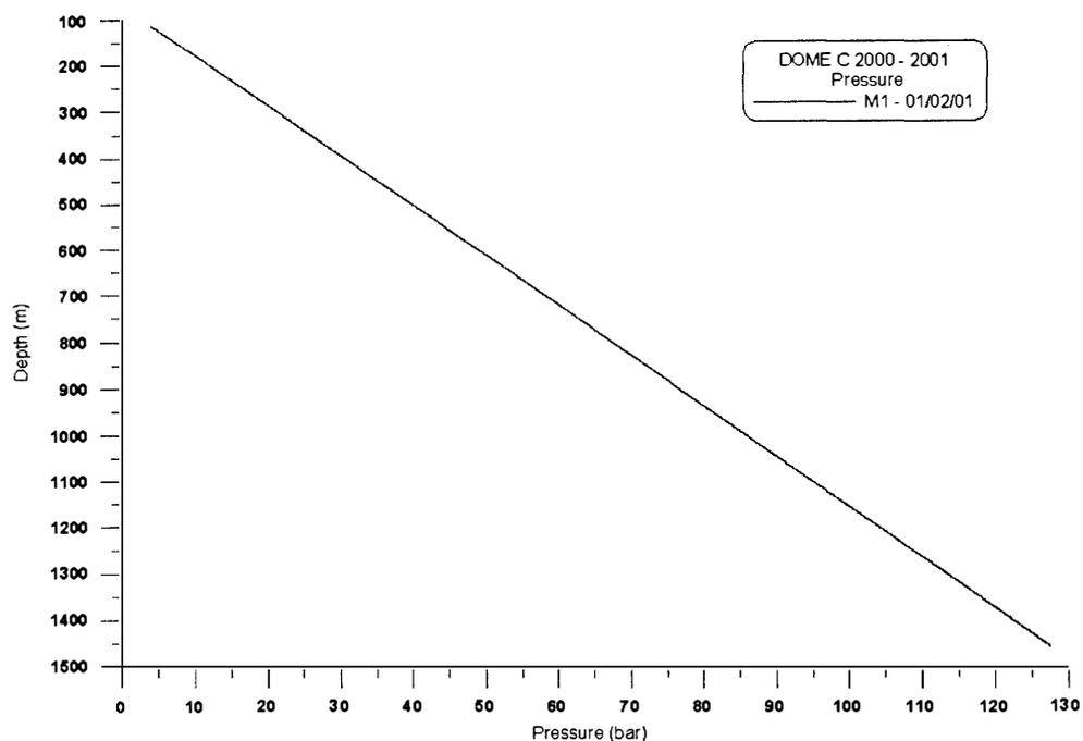
Fig. 11. Hole pressure measured in the Dome C second hole in 2001.
