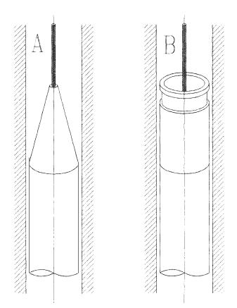
Fig. 2. Schematic of the ice core drill upper end: A-not recommended; B-recommended; details in the text.
