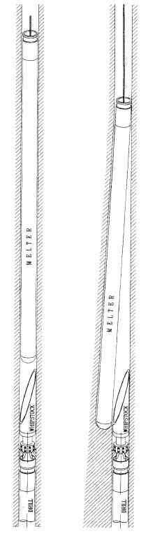
Fig. 4. Application of whipstock for passing object (drill) in the borehole.
