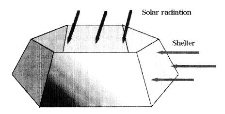
Fig. 1. A standard ITEX hexagonal open-top chamber (OTC). In the Latnjajaure set of OTCs, all panels are 60 cm wide at base and 40 cm high; the inclination of the walls is 73°.
