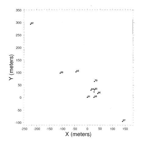
Fig. 5. The local control network around the Ny-Ålesund VLBI antenna. The VLBI antenna position (its azimuth axis) is marked by an open circle and a letter V. The pillars are marked with filled circle and the reference number used also in Table 1. The origin of the axis is pillar 91. The pillars 99 and 70 are not permanent and have been added using a tripod.
