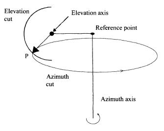
Fig. 2. A scheme of the motion of a generic point on the antenna during a rotation in azimuth and in elevation.
