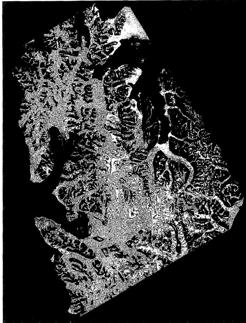
Fig. 2. Differential interferogramme over northwestern Spitsbergen from ERS-1 data recorded on ascending orbits the 17 and the 23 September 1991 (six days interval). The image is oriented to the North and covers the area of one complete ERS-1 scene ( 100 \times 120 km). Despite of the scale, clear fringes are visible on several glaciers on the eastern part of the image while due to the meteorological condition the western part is characterised by a low coherence and lack of fringes. Inverse conditions as well as radar features were observed between the 23 September and the 3 October and on the nine days interval interferogramme not presented here.
