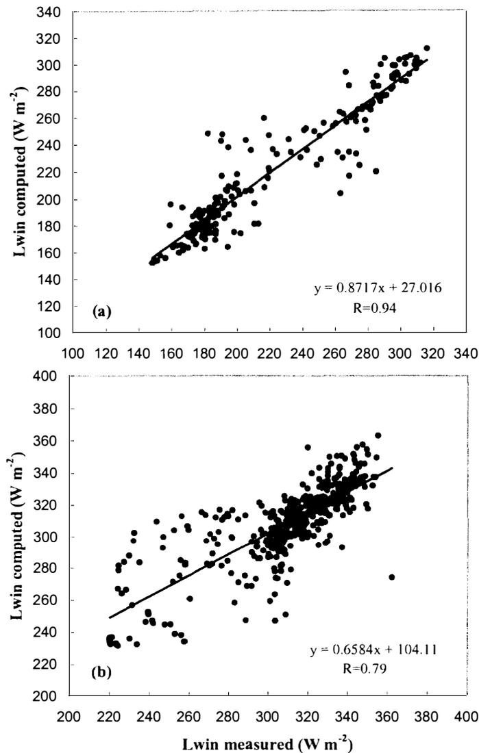
Fig. 1. Scatter plot between the longwave incoming radiation obtained through the Konzelmann *et al.* (1994) parameterization and that measured with the radiometer for (a) the ARTIST and (b) the LSF experiment.
