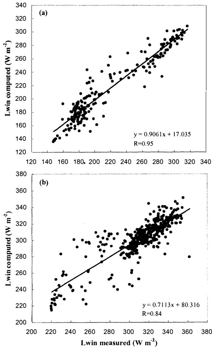
Fig. 2. Same as in Fig. 1 but with the longwave incoming radiation obtained through the De Rooy and Holtslag (1999) parameterization.
