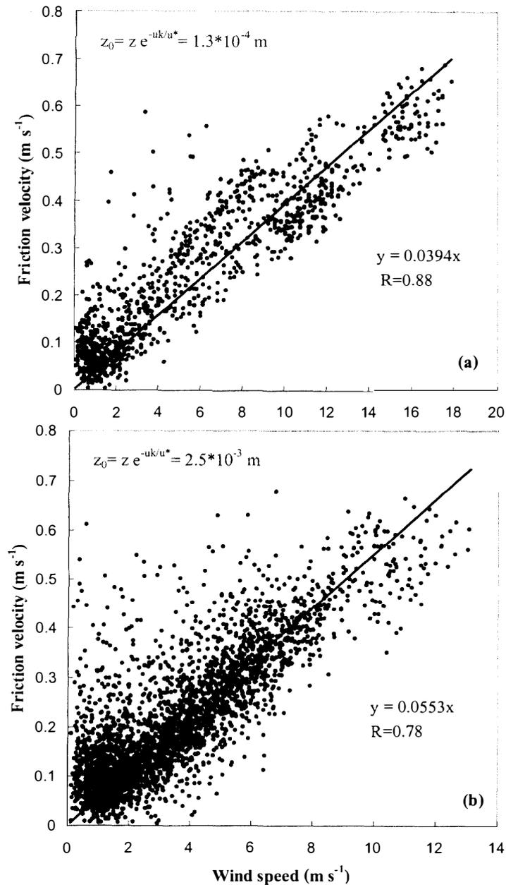
Fig. 3. Scatter plot between the friction velocity and the wind speed for (a) the ARTIST and (b) the LSF experiment.
