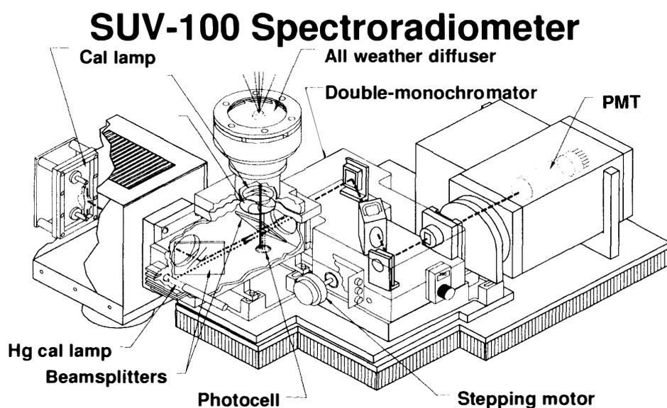
Fig. 1. SUV-100 pictorial diagram. The SUV-100D (e.g. Valdivia) is a redesigned version, with similar elements plus other enhancements.
