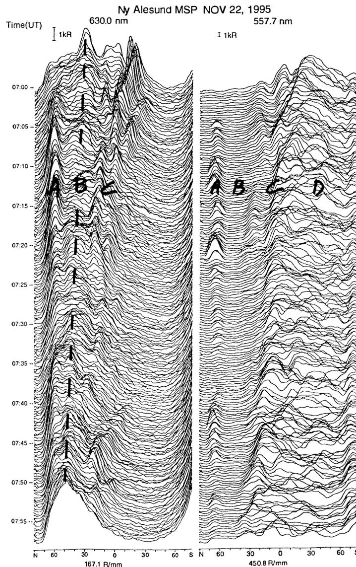
*Fig. 8. Meridian scanning photometer records of auroral emissions from 22 November 1995 are plotted as in Figs. 6 and 7. During this event several intensity maxima -labeled A, B, C and D- are observed. The different forms represents signatures of the different layers presented in Fig. 3. Notice the variations in first structure and dynamics. For further details, see the text.*
