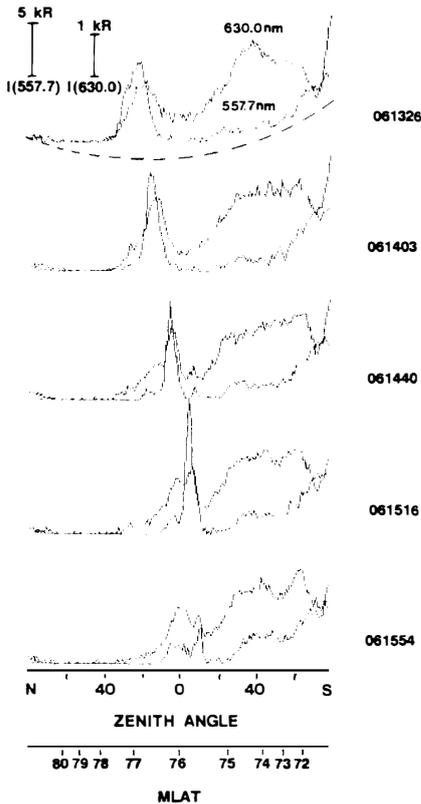
Fig. 6. North-south meridian photometer scans at Ny-Ålesund, Svalbard ( $75.4^\circ$  MLAT) at wavelengths 630.0 and 557.7 nm plotted as function of time (UT) and zenith angle. Intensity scales are given in the upper left corner. MLT is approximately three hours ahead of UT. Thus, the recordings shown are close to 0920 MLT. By assuming an altitude of 250 km the zenith angles are converted to MLAT in the lowest scale. During this event, both the cusp and the mantle regions are observed.
