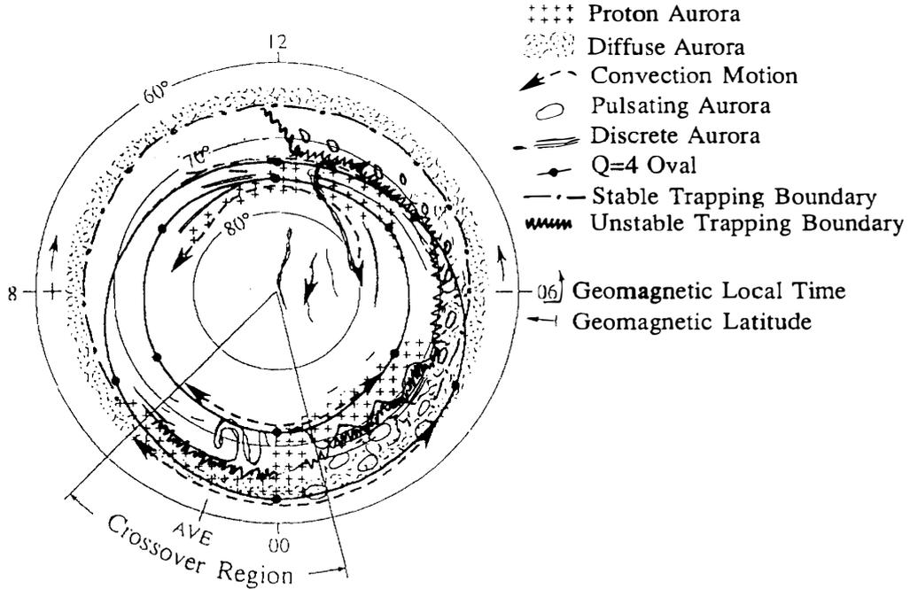
Fig. 5. This map of the northern hemisphere - in magnetic time and latitude - is based on extensive ground and rocket observations during the SCIFER rocket launch. The locations, widths and large scale changes are indicated. Such a detailed map could never be obtained without a net of advanced ground measurements.
