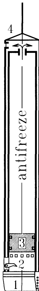
Fig. 1. Schematic of the antifreeze thermal electrical drill (ATED): 1) drilling bit; 2) core catchers; 3) piston; 4) cable.
