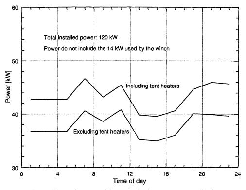
Fig. 7. Electrical power used during the day for camp operation. Winch power (14 kW) is not included The capacity of the generator is 65 kW, and the total installed power was 120 kW.
