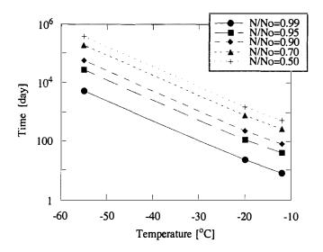
Fig. 4. Storage temperature and time period diagram of air-hydrate dissociation in ice. Each line represents a dissociation ratio of air-hydrate crystals from 1 to 50%. If a deep ice core, which includes air-hydrate crystals, is stored at −20°C for 90 days, this diagram says that about 4% of the crystal will dissociate.
