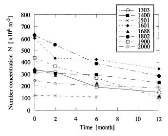
Fig. 3. Change of the number concentration of air-hydrate crystals in Dye-3 ice cores with time period at  $-12^{\circ}C$  (SHIGESATO, 1985).
