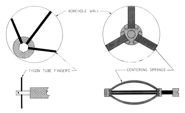
Fig. 5. Logger in borehole.
