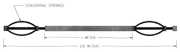
Fig. 4. The short logger with centering springs.
