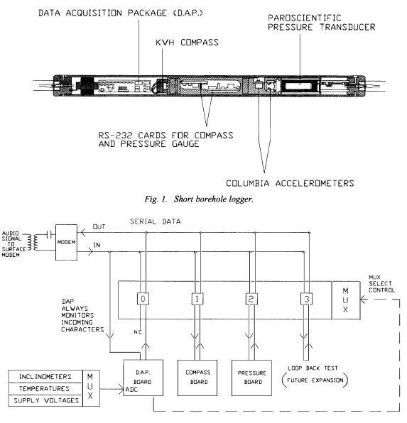
Fig. 2. Block diagram of DAP interconnections.
