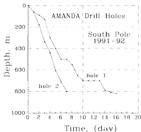
Fig. 1. Drill depth vs. time.
