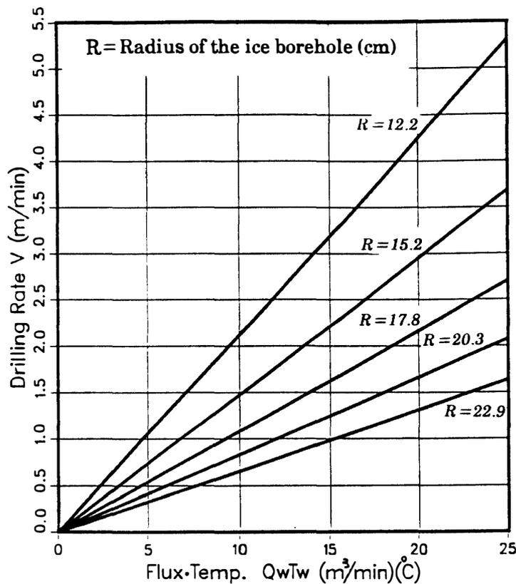
Fig. 6. Graph of flux temperature versus drilling rate.
