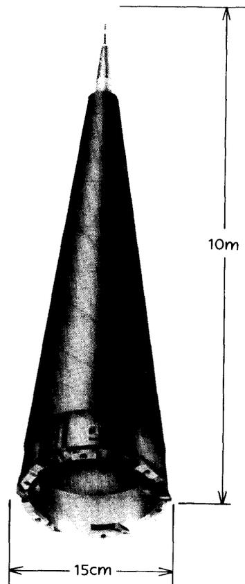
*Fig. 7. Conceptual drawing of hot-water mechanical drill.*
