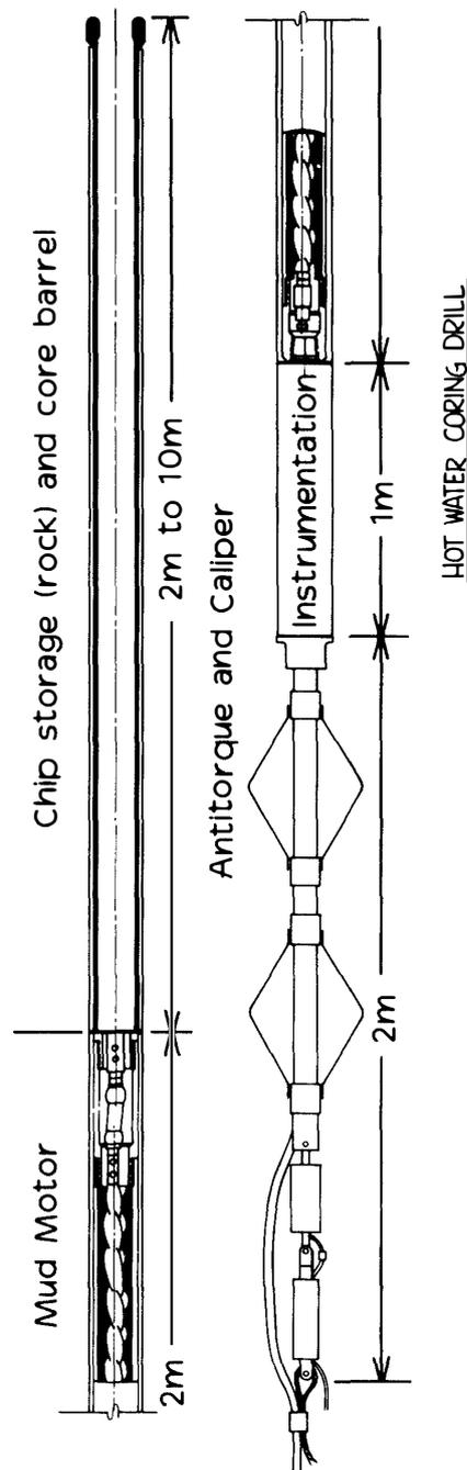
Fig. 5. Cross-section of hot-water coring drill.
