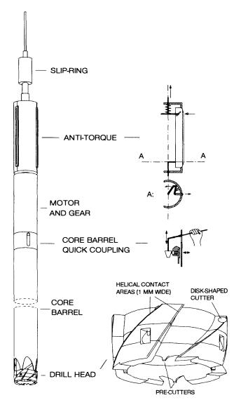
Fig. 2. Drill and drill head. The three skates of the anti-torque section are retracted while hoisting the drill. During drilling the upper part of the skates is activated by a decrease in cable tension and the lower part is forced out by torque.
