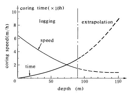
Fig. 4. Penetration performance of the BZXJ drilling system.
