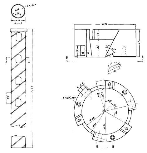
Fig. 2. Structure of the core barrel.
