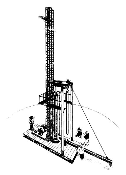
Fig. 4. Tower and surface equipment for the PICO 13.2 cm ice coring drill.
