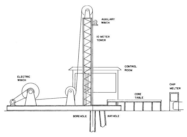
Fig. 3. Possible future design of surface handling equipment for the PICO 13.2 cm ice coring drill.
