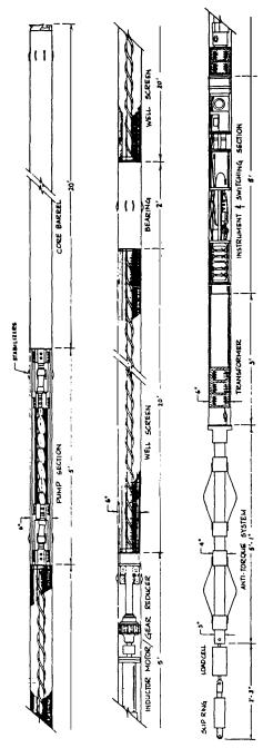
Fig. 1. Cross-sectional drawing of the existing PICO 13.2 cm ice coring drill.
