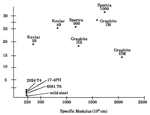
Fig. 2. Tensile strength of various drill cable materials.
