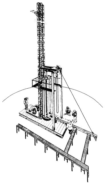
Fig. 1. PICO 13.2 cm ice core drill handling system.
