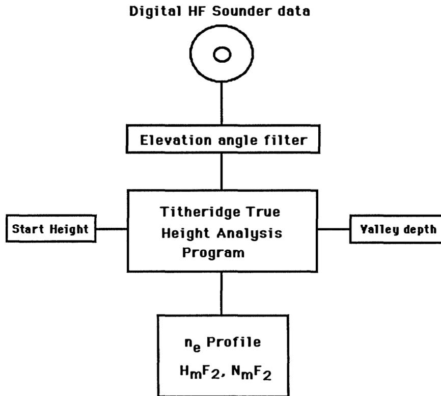
Fig. 2. A schematic diagram illustrating the methods by which the observational data have been analyzed.
