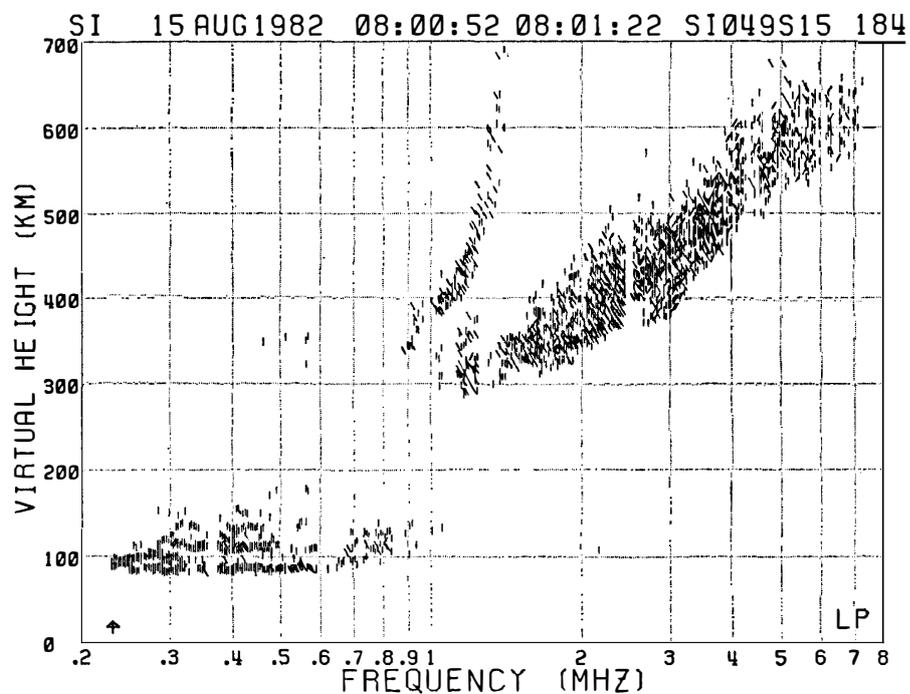
Fig. 3. An ionogram recorded at Siple Station, Antarctica on August 15, 1982 at 0800:52 UT. Echoes from the ionospheric trough occur between 1.0 and 1.4 MHz. Echo polarization is denoted by the orientation of the graphics symbol.
