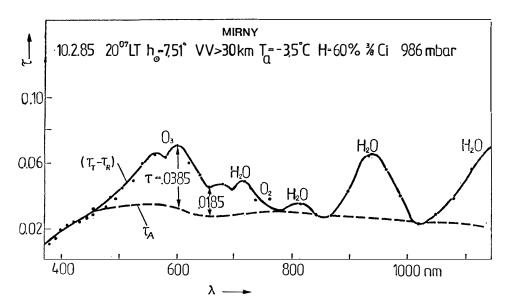
Fig. 1. Diagram showing the graphical smoothing of the  $(\tau_T - \tau_R)$ -curve to eliminate the optical thickness of water vapour, ozone and oxygen. VV: visibility,  $T_a$ : air temperature, H: relative humidity, Ci: Cirrus clouds.
