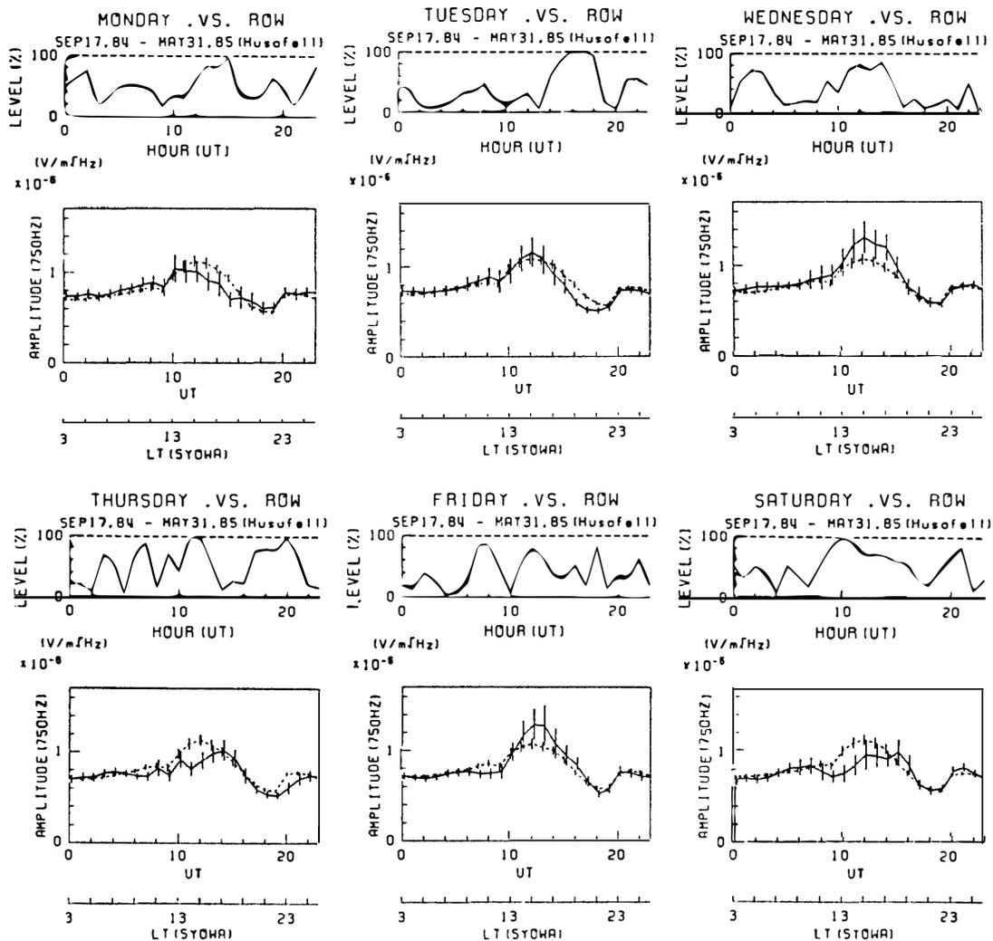
Fig. 5. Averaged daily variation of electric field intensity at a frequency of 750 Hz at Husafell, on each day of the week and on ROW.
