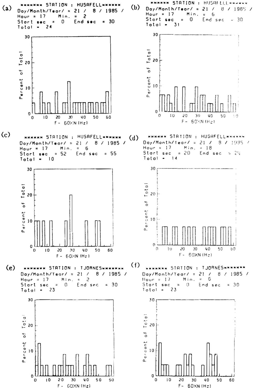
Fig. 11. Deviation in frequency of the harmonic line structures in the VLF spectra below 2 kHz, observed at Husafell and Tjörnes, from the higher harmonics of 60 Hz.
