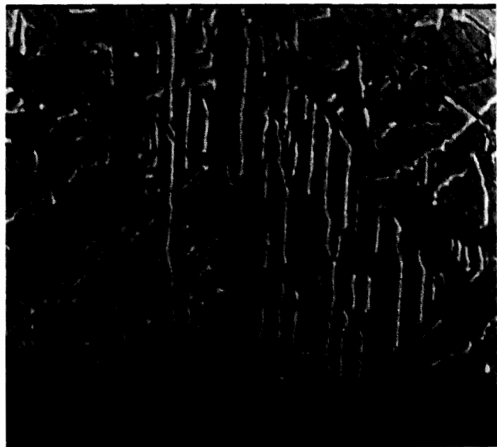
Fig. 3. SEM photograph of shock-hatched kamacites. Small fine bristles and wide "bristles" which consist of several fine bristles are seen. Scale bar: 10 \mu .
