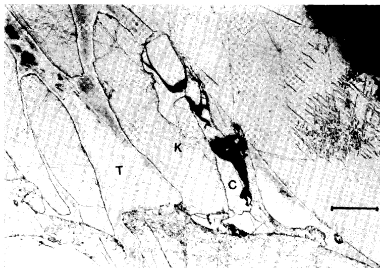
Fig. 4. Partially recrystallized kamacites (lower) within the kamacite. They appear beside cohenites and taenites. K: kamacite, T: taenite, C: cohenite. Scale bar: 100 \mu .
