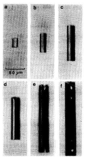
Fig. 1. Columnar ice crystal grown in air at  $1.0 \times 10^5$  Pa at  $-30^{\circ}C$  and 1.4% supersaturation. (a) 0, (b) 12.0, (c) 39.3, (d) 50.1, (e) 84.3, (f) 97.3 min.
