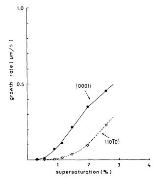
Fig. 4. Supersaturation dependence of the normal growth rates of the  $\{0001\}$  and  $\{10\overline{1}0\}$  faces of a columnar ice crystal grown in air at  $4.0 \times 10$  Pa at  $-30^{\circ}C$ .
