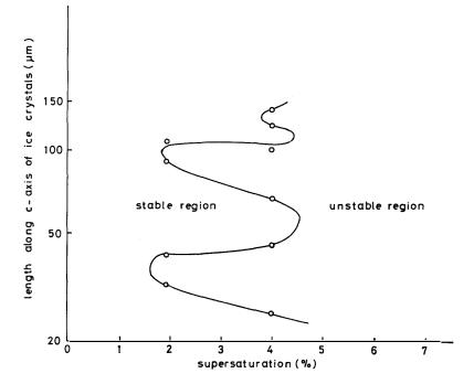
Fig. 3. Instability limit of the  $\{10\overline{1}0\}$  face of columnar ice crystals grown in air at  $3.3 \times 10^4$  Pa at  $-30^{\circ}C$ .
