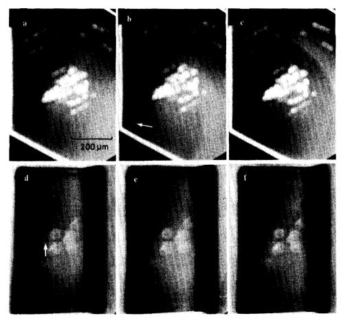
Fig. 5. Surface microtopography of the  $\{0001\}$  and  $\{10\overline{1}0\}$  faces of ice crystals grown in air at  $4.0 \times 10$  Pa at  $-30^{\circ}$ C. The upper and lower crystals show the  $\{0001\}$  and  $\{10\overline{1}0\}$  faces, respectively. (a) 0, (b) 5, (c) 10 s; (d) 0, (e) 2, (f) 4 s.
