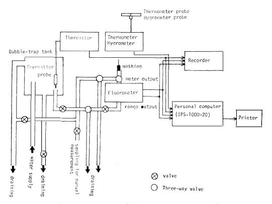
Fig. 1. Schematic representation of the continuous measuring-recording system of the surface chlorophyll a employed for the JARE-26 (1984/85).
