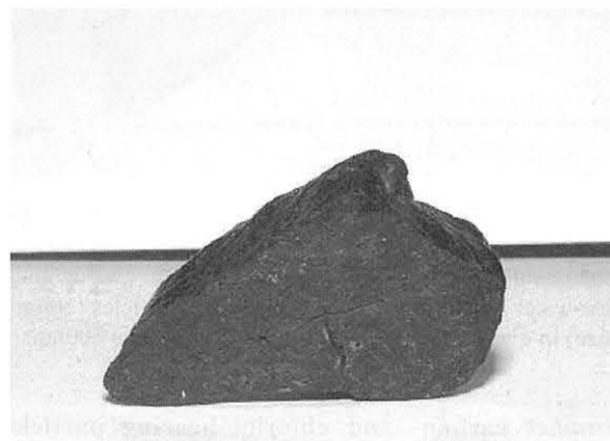
Figure 1. Handspecimen of NWA 5011 meteorite. The abundant shock veins network is clearly seen.
