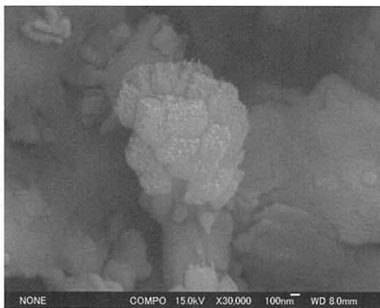
Fig.3. High-resolution (FE-SEM) electron micrographs of fine carbon-bearing particles on the Takamatsu drilled breccias sample of 950m in depth formed by impact on sea-carbonates. Previous results on impact on granitic rocks have few calcite or carbon-bearing rocks, though there are different sea-bottom rocks with carbon. Bar is 100nm in scale [5].
