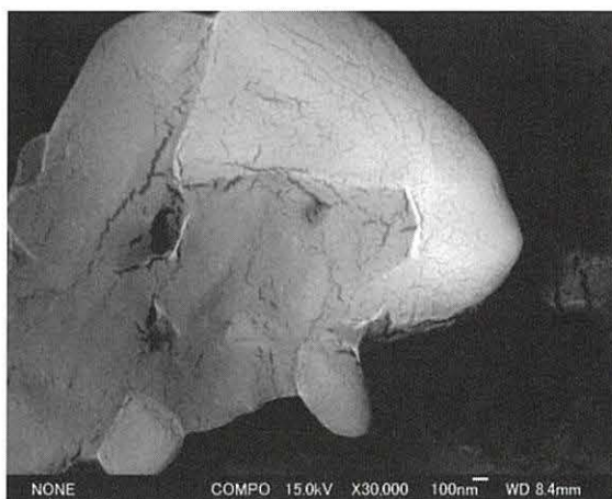
Fig.1. The ASEM in-situ electron-micrograph of the LDSG tektite sample with C, Mg, Al, K, Cr and Fe (back) [4], together with Na and Cl (white grains). Impact halites are aggregates of nano-particles (10nm in size). The scale bar is 100nm.
